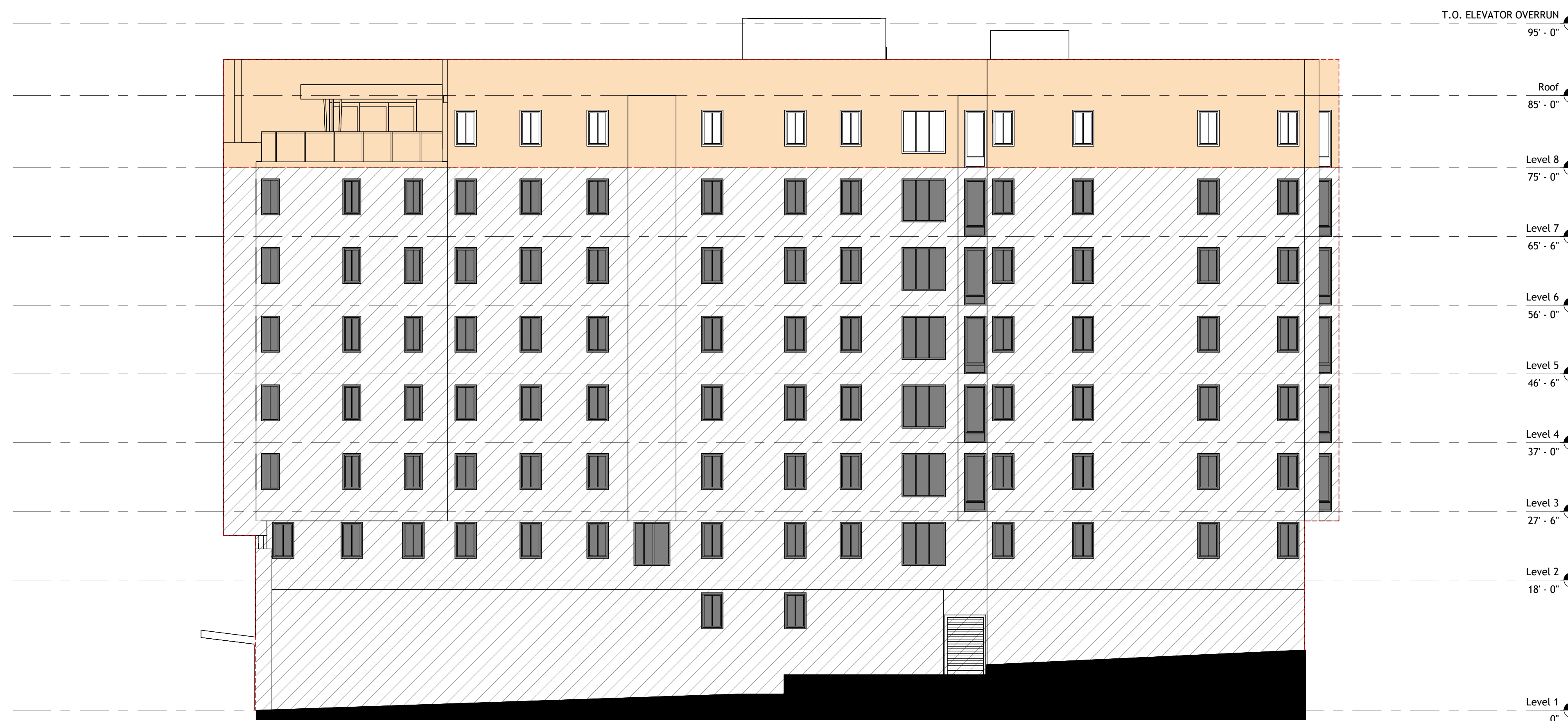
2 SOUTH ELEVATION - BIRD SAFE GLAZING 3/32" = 1'-0"
