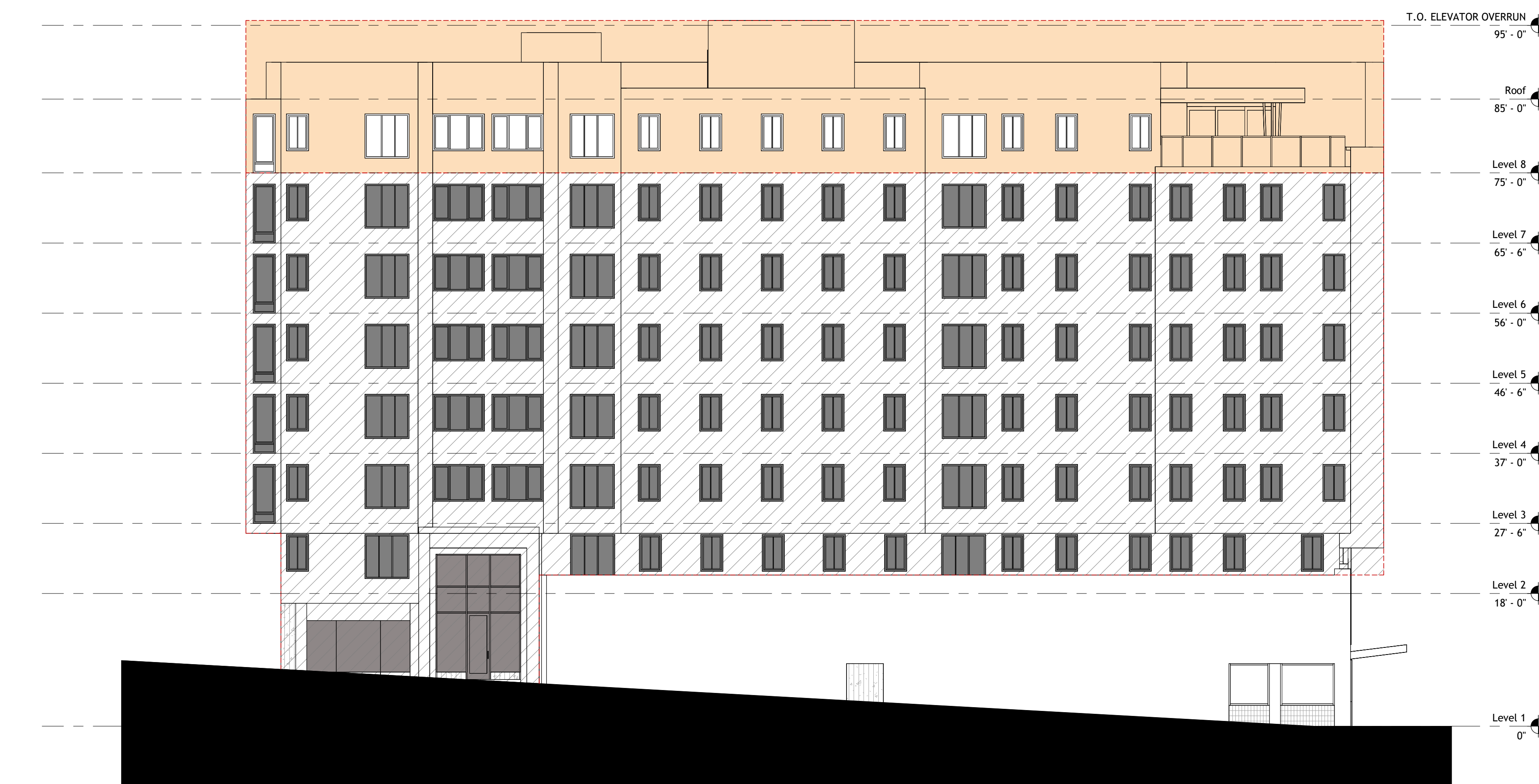
1 NORTH ELEVATION - BIRD SAFE GLAZING 3/32" = 1'-0"
