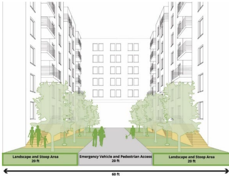
Figure 10. Diagram of Access Drive through Development Area B (Illustrative Concept)
