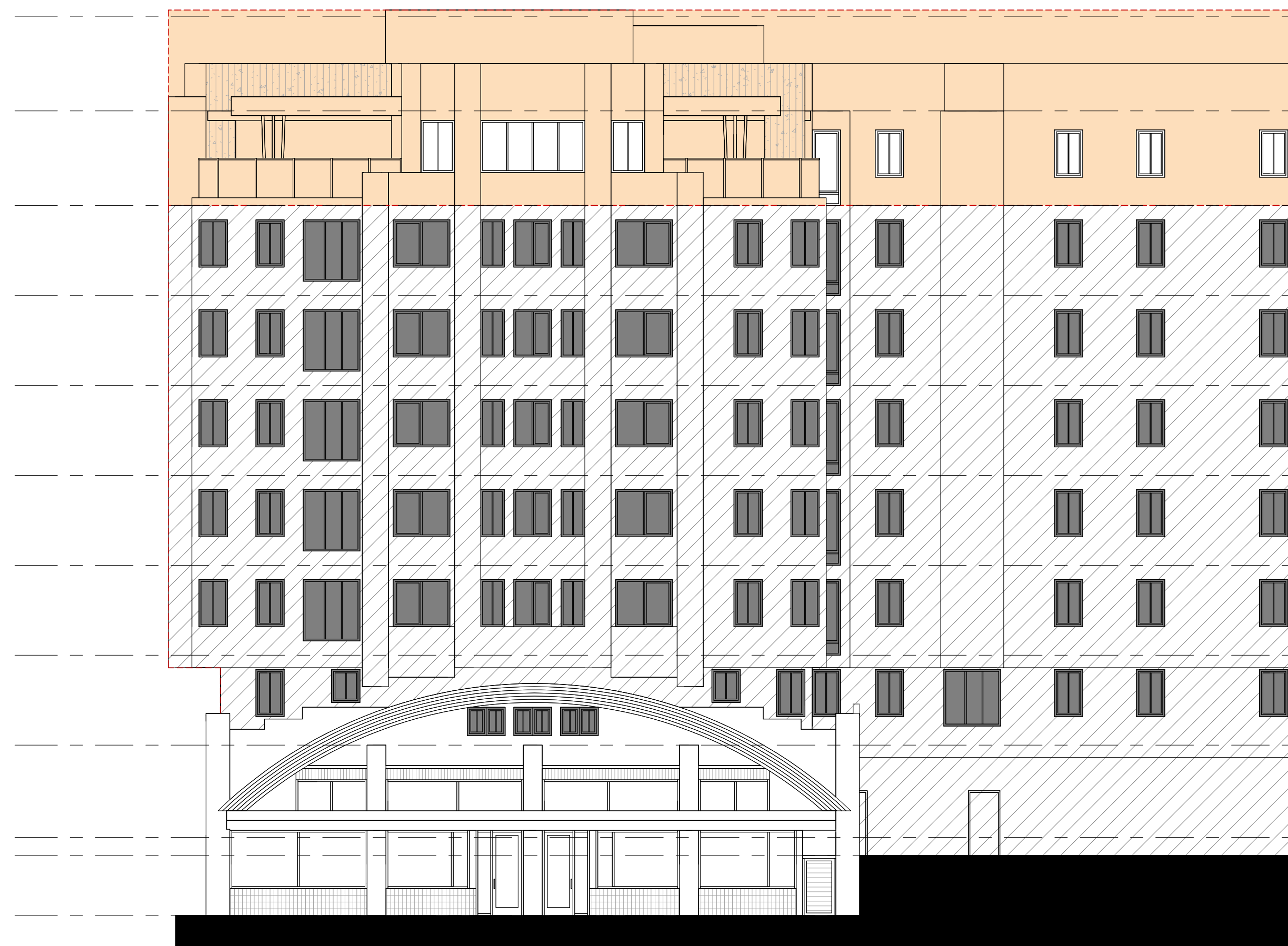
2 WEST ELEVATION - BIRD SAFE GLAZING 3/32" = 1'-0"
