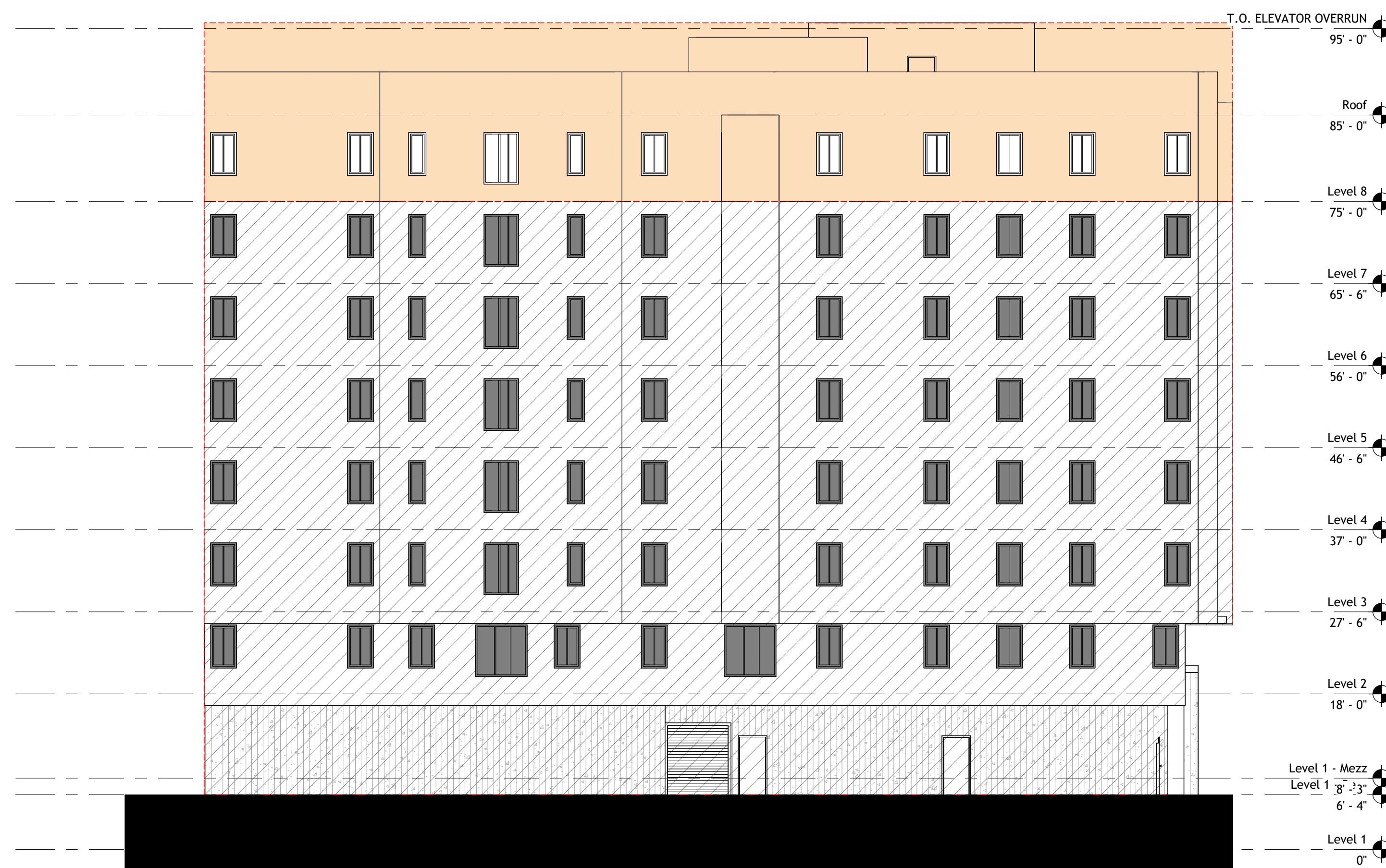
2 WEST ELEVATION - BIRD SAFE GLAZING 3/32" = 1'-0"
