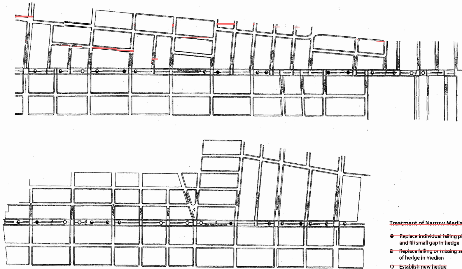
Figure 28: Treatment of Narrow Medians
