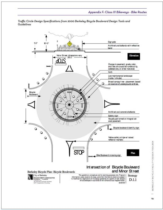
Berkeley's Design Specifications for Traffic Circles include a broad canopy tree in the center of the circle. The recommendation to include a tree is illustrated in 2 places: at the top, via the elevation drawing and in the middle, via the aerial view.
