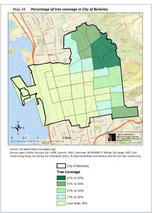
Map illustrating the distribution of tree coverage in Berkeley. The densest tree coverage is located in the hills in east Berkeley while the fewest trees are in the west and south, where a majority of the traffic circles are located. The LHMP recommends expanding tree coverage in Berkeley to help mitigate the UHIE (Urban Heat Island Effect) and the anticipated increase in extreme heat days, as well as to safeguard public health. Expanding tree coverage can also address historical inequities.
