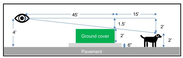
Figure 2 Vertical sight line measurement
