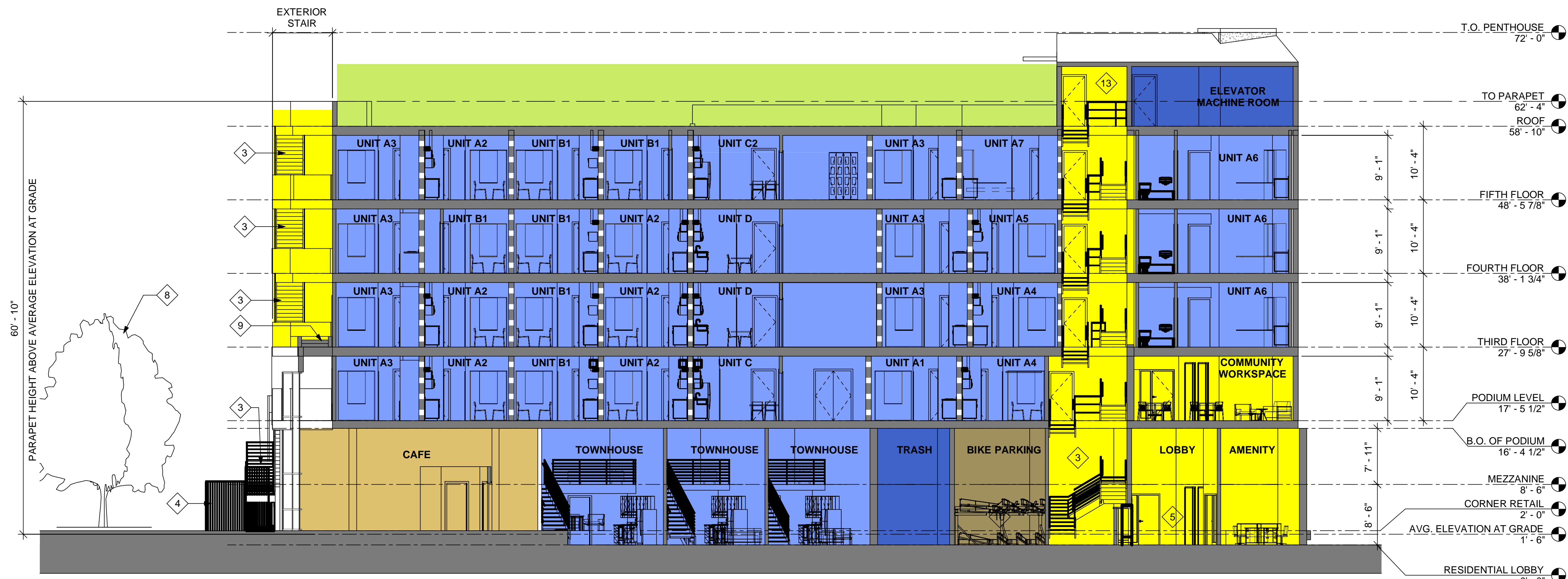
① LONGITUDINAL SECTION THROUGH UNITS 1/8" = 1'-0"
