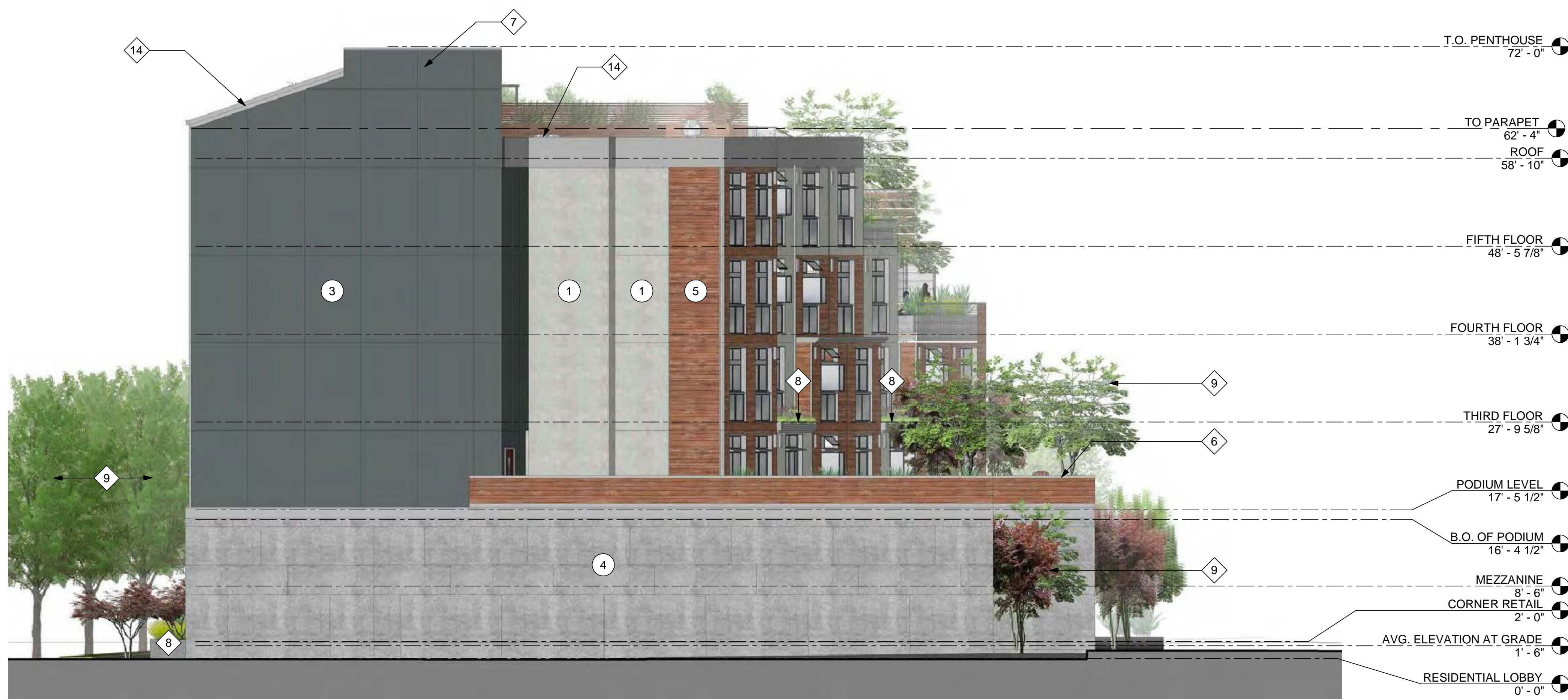
② EXTERIOR ELEVATION SOUTH 1/8" = 1'-0"
