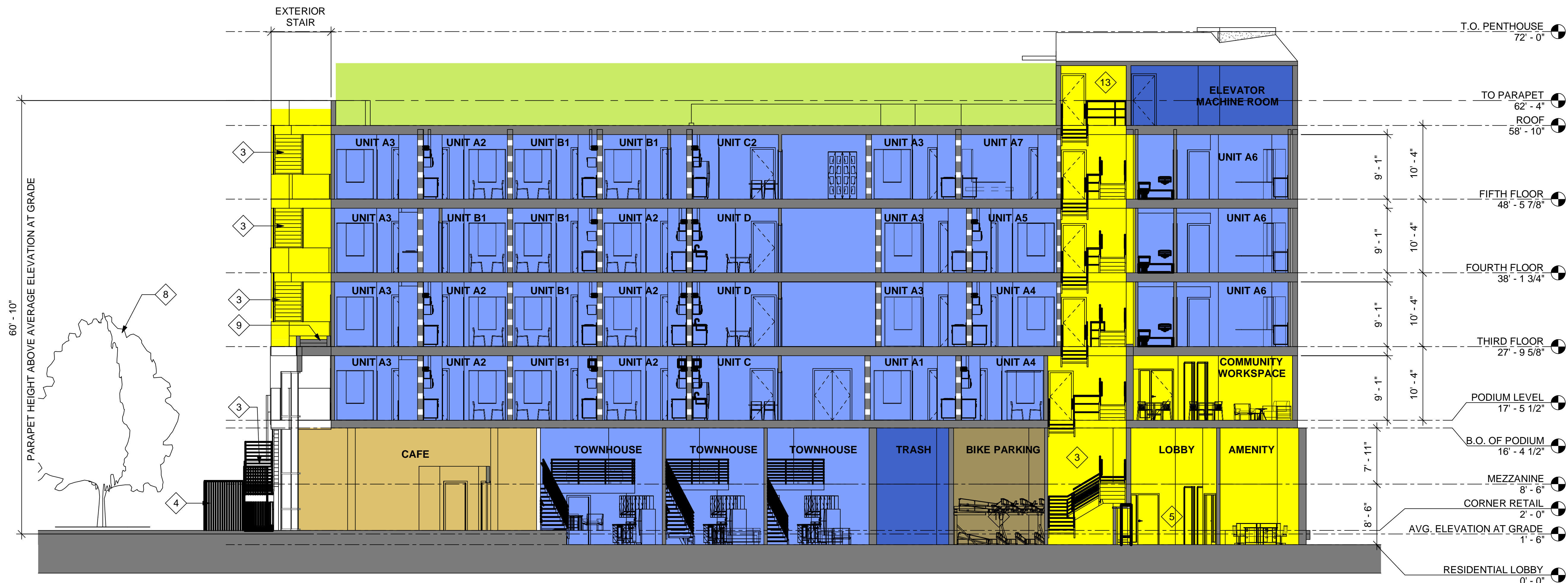
1 LONGITUDINAL SECTION THROUGH UNITS 1/8" = 1'-0"
