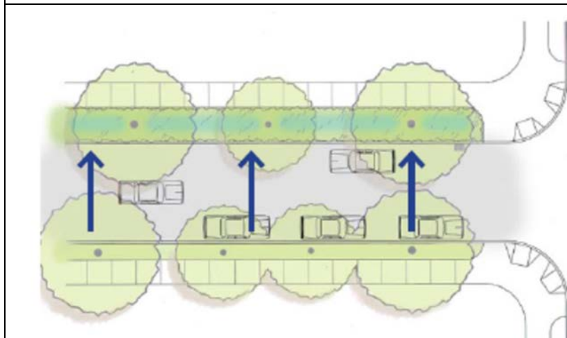
Figure C-3. Side Shed Street Profile. Side shed streets are designed to shed all water to one side of the street. GI facilities would be located on the downslope side.
