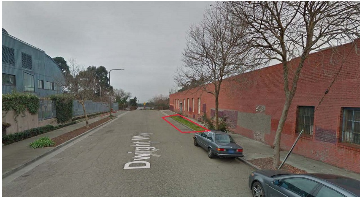
Figure 31 – Extension and retrofit of existing sidewalk planter strips into bioretention features may be feasible on Dwight Way between Fourth Street and the UPRR ROW.
