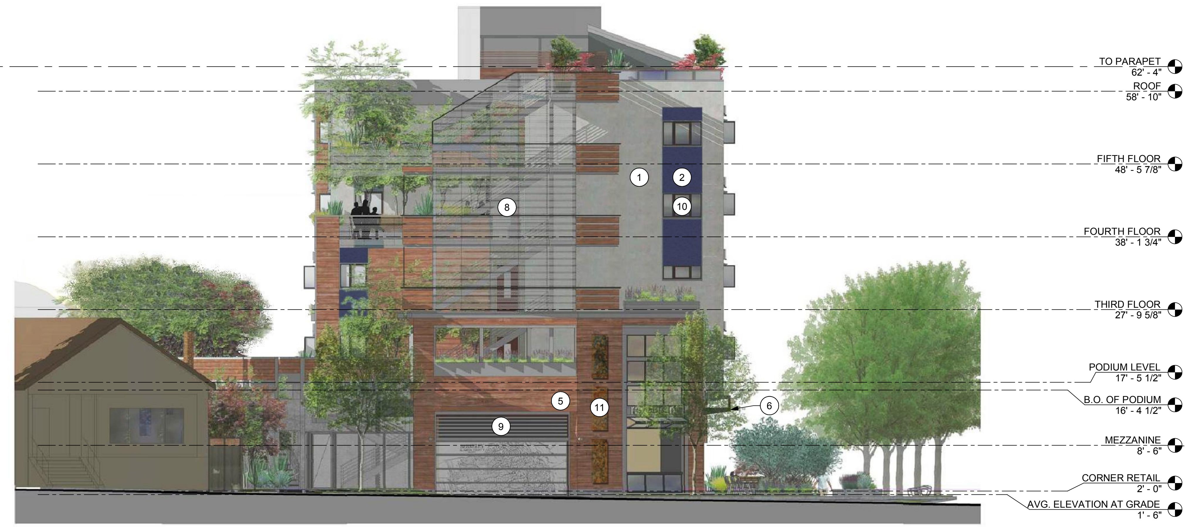
2 EXTERIOR ELEVATION - NORTH 1/8" = 1'-0"
