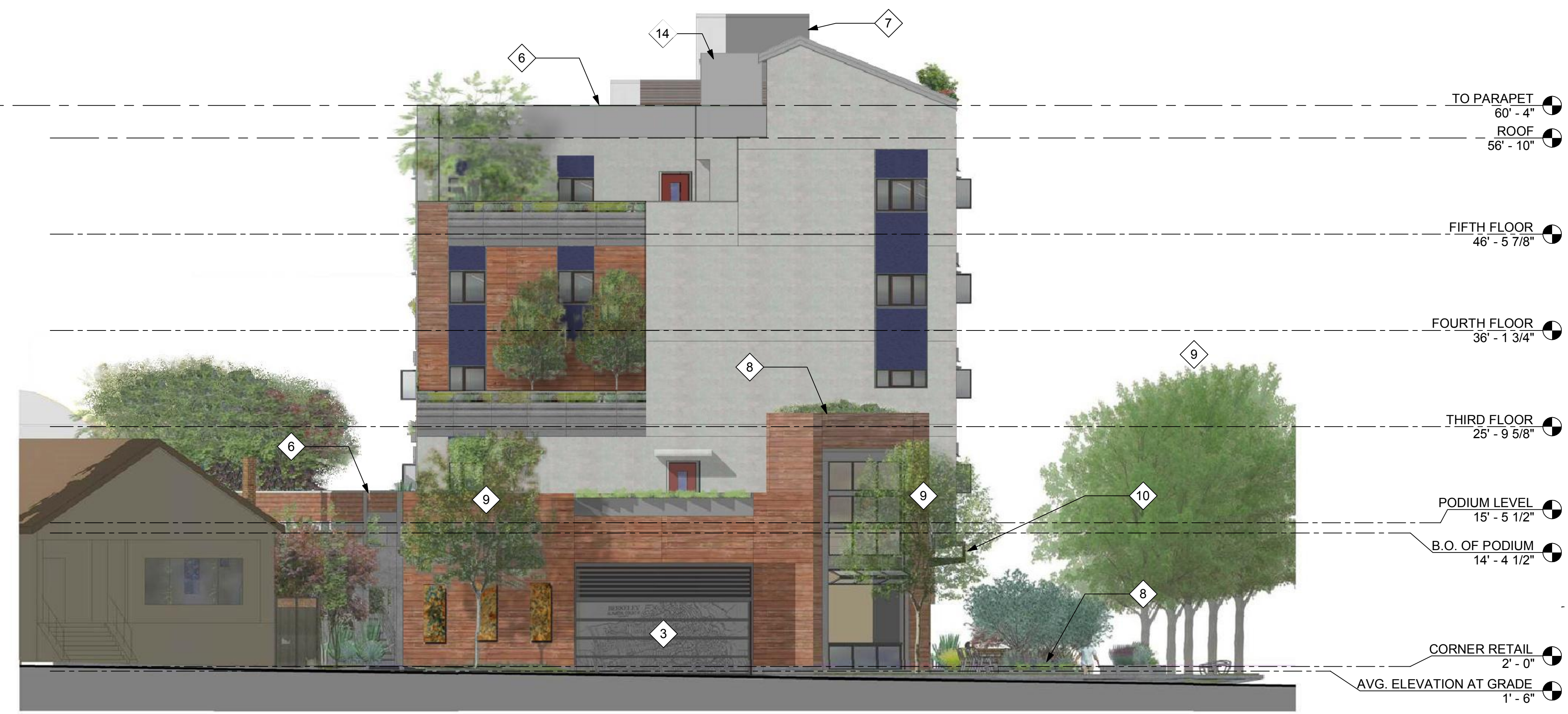
2 EXTERIOR ELEVATION - NORTH 1/8" = 1'-0"
