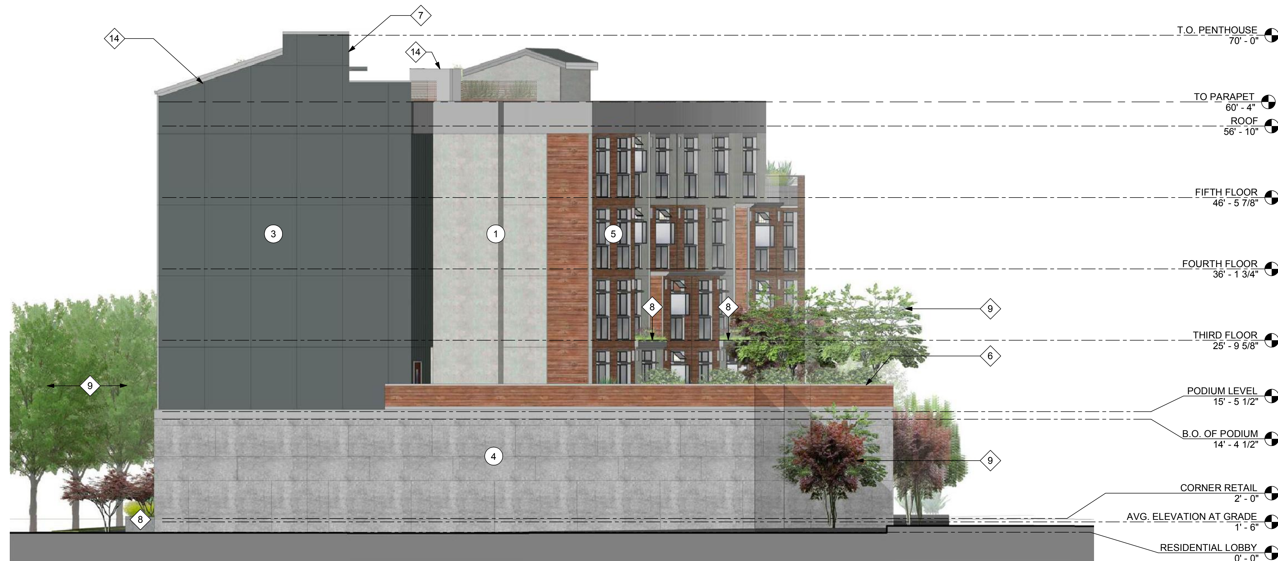
2 EXTERIOR ELEVATION SOUTH 1/8" = 1'-0"
