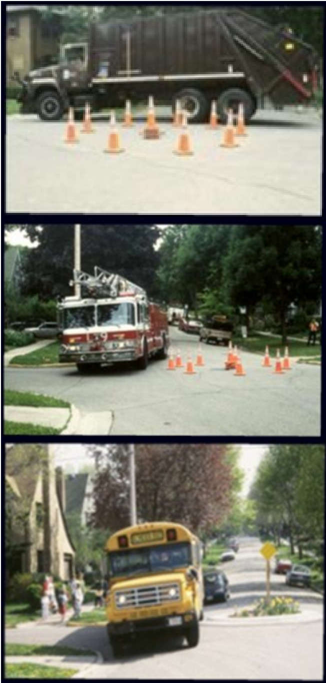
Figure 11 testing of traffic circles for large vehicles
