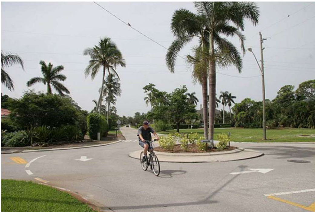
Figure 17 Bicyclist passing through traffic circle with mountable curb, low ground cover, low directional signs, tall and slender trees, painted splitter islands, no stop signs, and one visible crosswalk set back from the circle.
