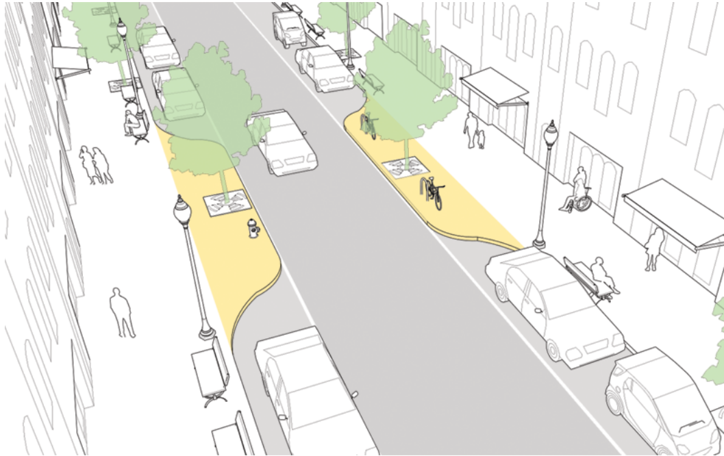
Figure 29 NACTO recommends planting trees on curb extensions aligned to the parking lane to narrow the overall profile of the roadway and reduce traffic speed
