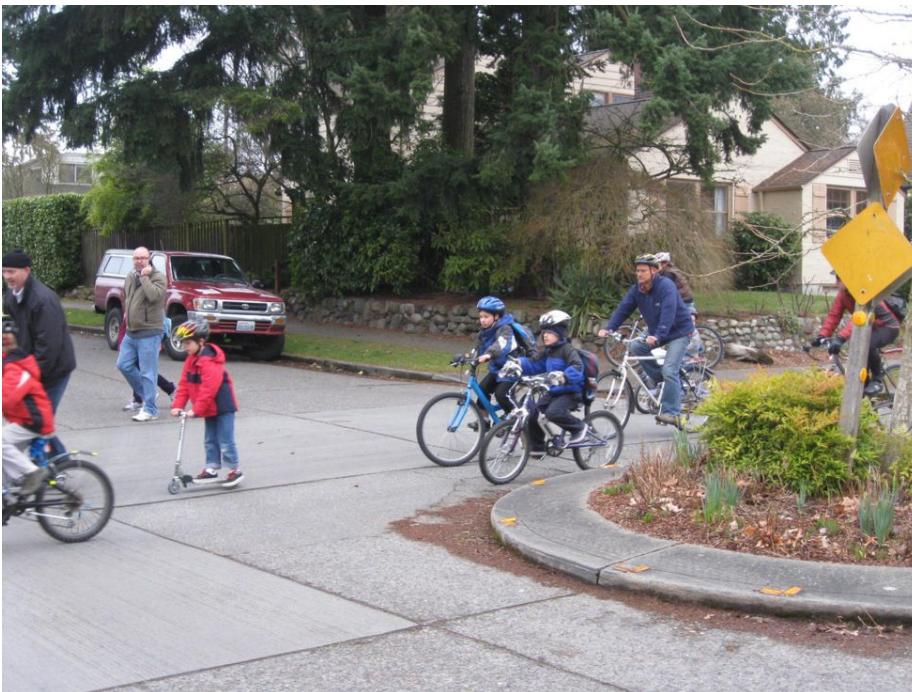
Figure 24 Image of a neighborhood traffic circle in the NACTO Urban Street Design Guide featuring low ground cover and no trees.
