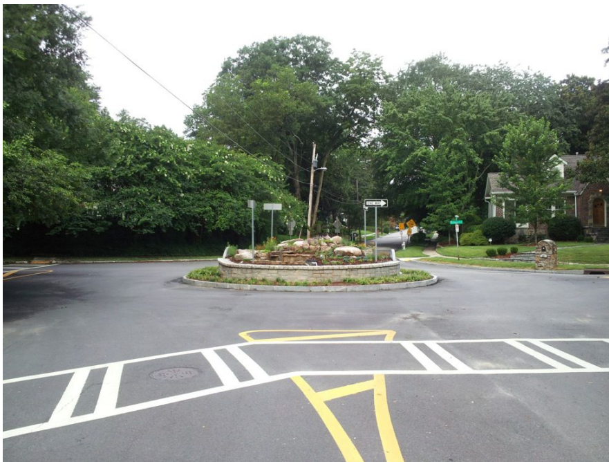
Figure 26 Image of a neighborhood traffic circle in the NACTO Urban Street Design Guide featuring painted splitter islands, low ground cover, and no trees.
