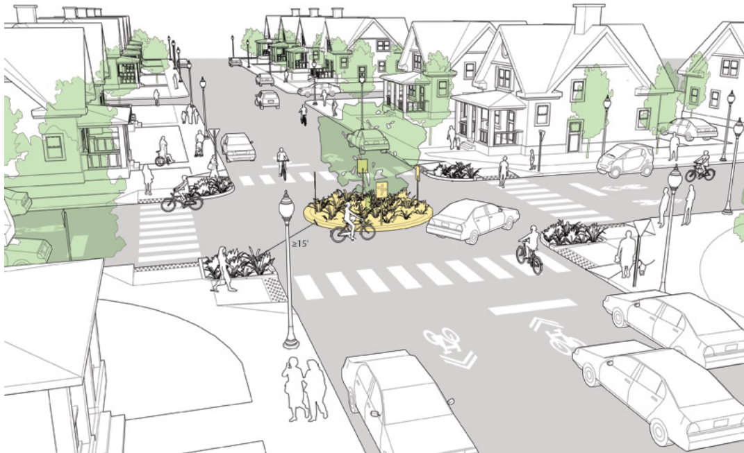
Figure 19 Conceptual rendering of a neighborhood traffic circle in NACTO's Urban Street Design Guide.
