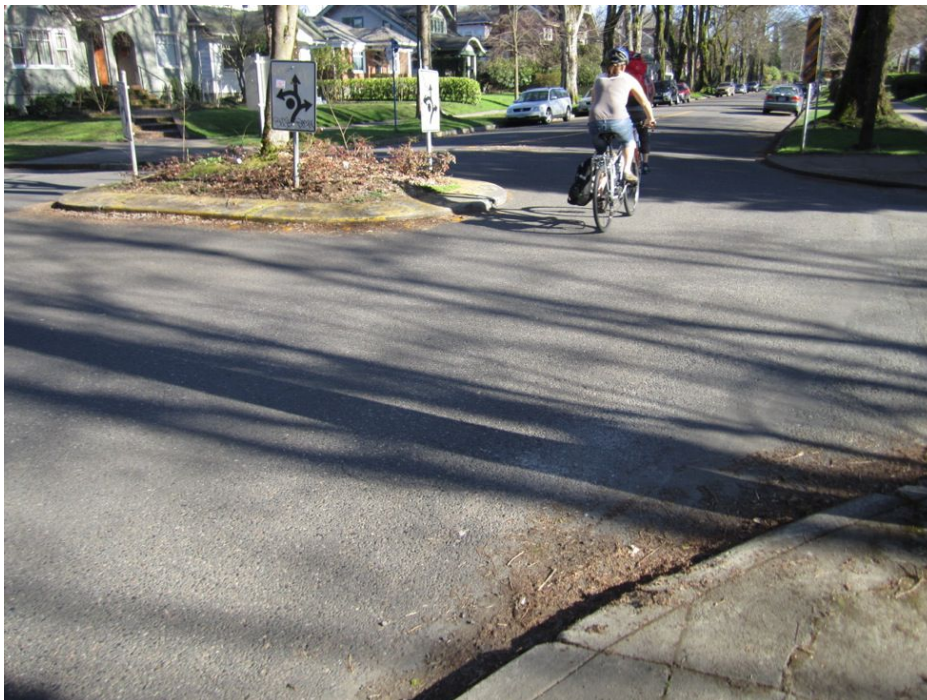
Figure 22 Image of a neighborhood traffic circle in the NACTO Urban Street Design Guide featuring low ground cover and no trees.
