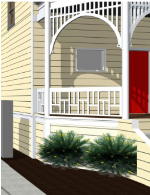
Figure 8: restored wood filigree arches at porch
