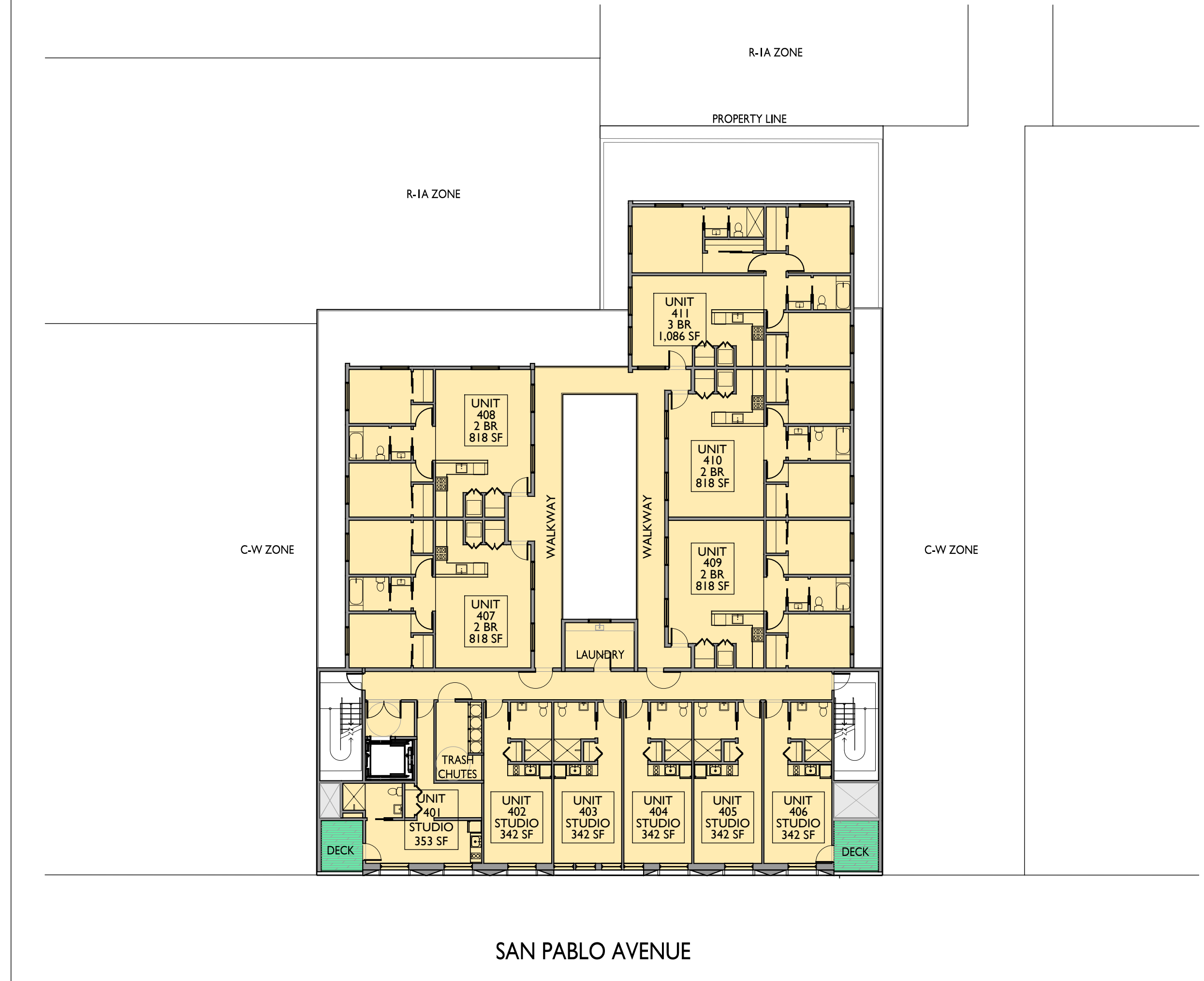
3 PROPOSED PROJECT - FOURTH FLOOR PLAN SCALE 1/16" = 1'-0"
