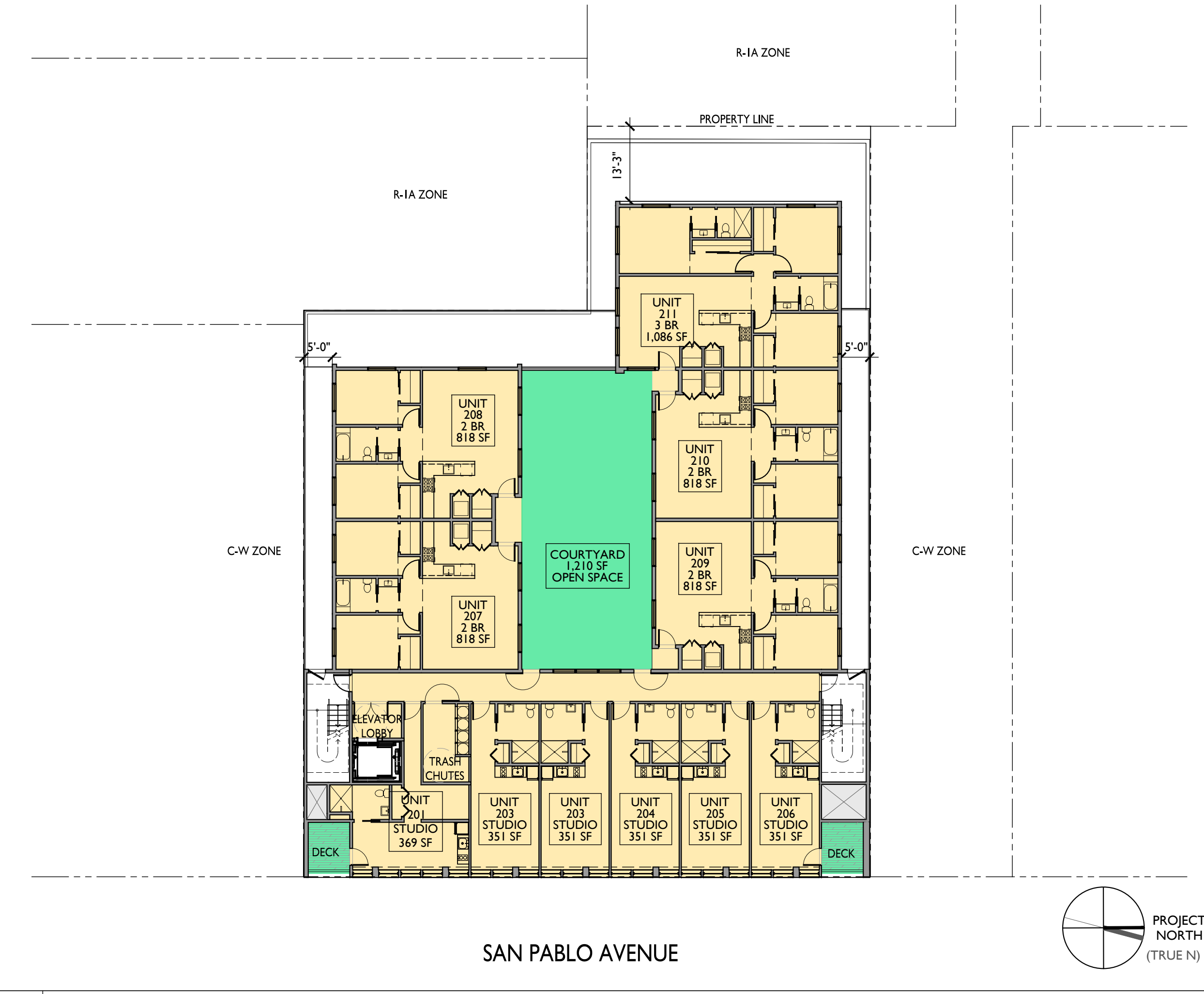
1 BASE PROJECT - SECOND FLOOR PLAN SCALE 1/16" = 1'-0"
