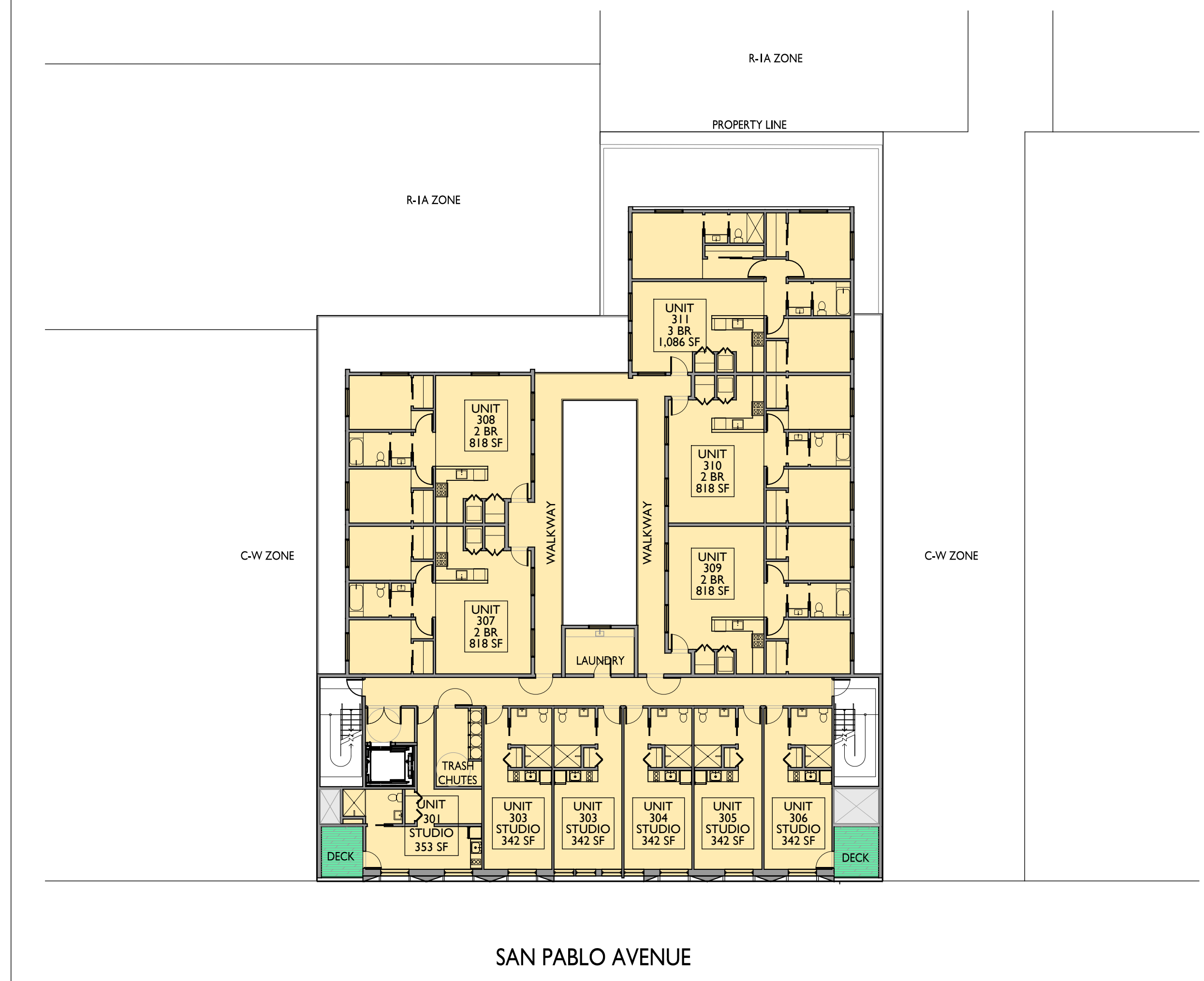
4 PROPOSED PROJECT - THIRD FLOOR PLAN SCALE 1/16" = 1'-0"
