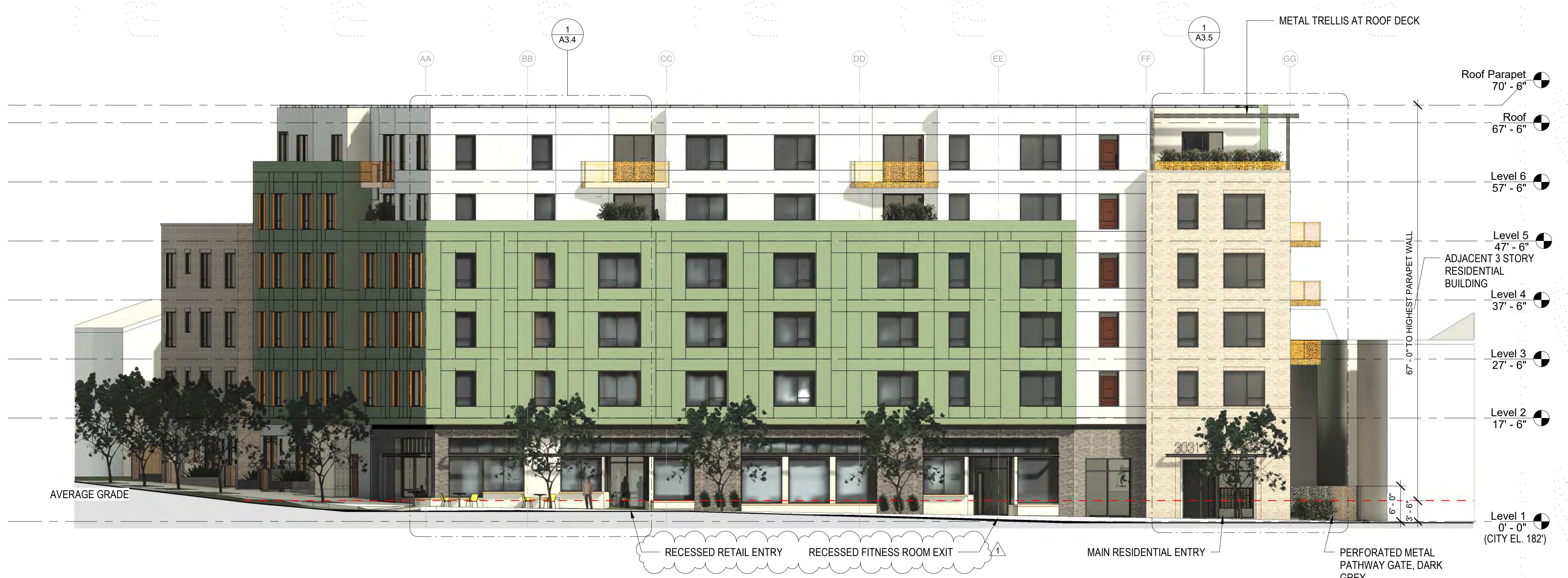
2 WEST ELEVATION - TELEGRAPH AVENUE 3/32" = 1'-0"
