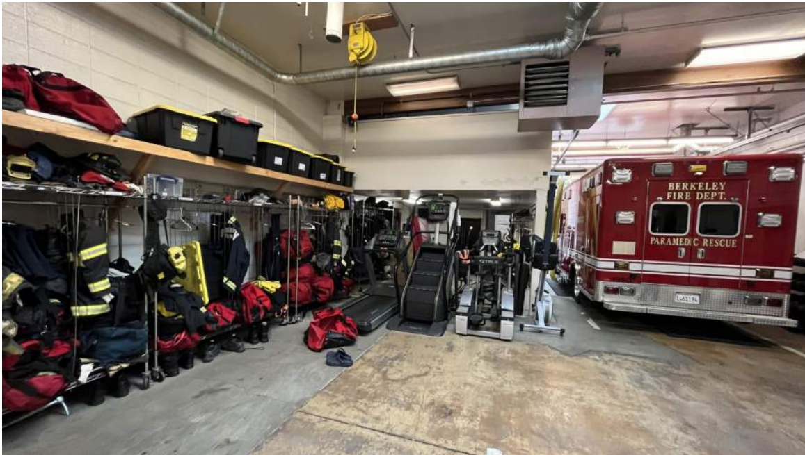
Turnouts, exercise equipment, and apparatus all in the same space do not meet current best practices.
