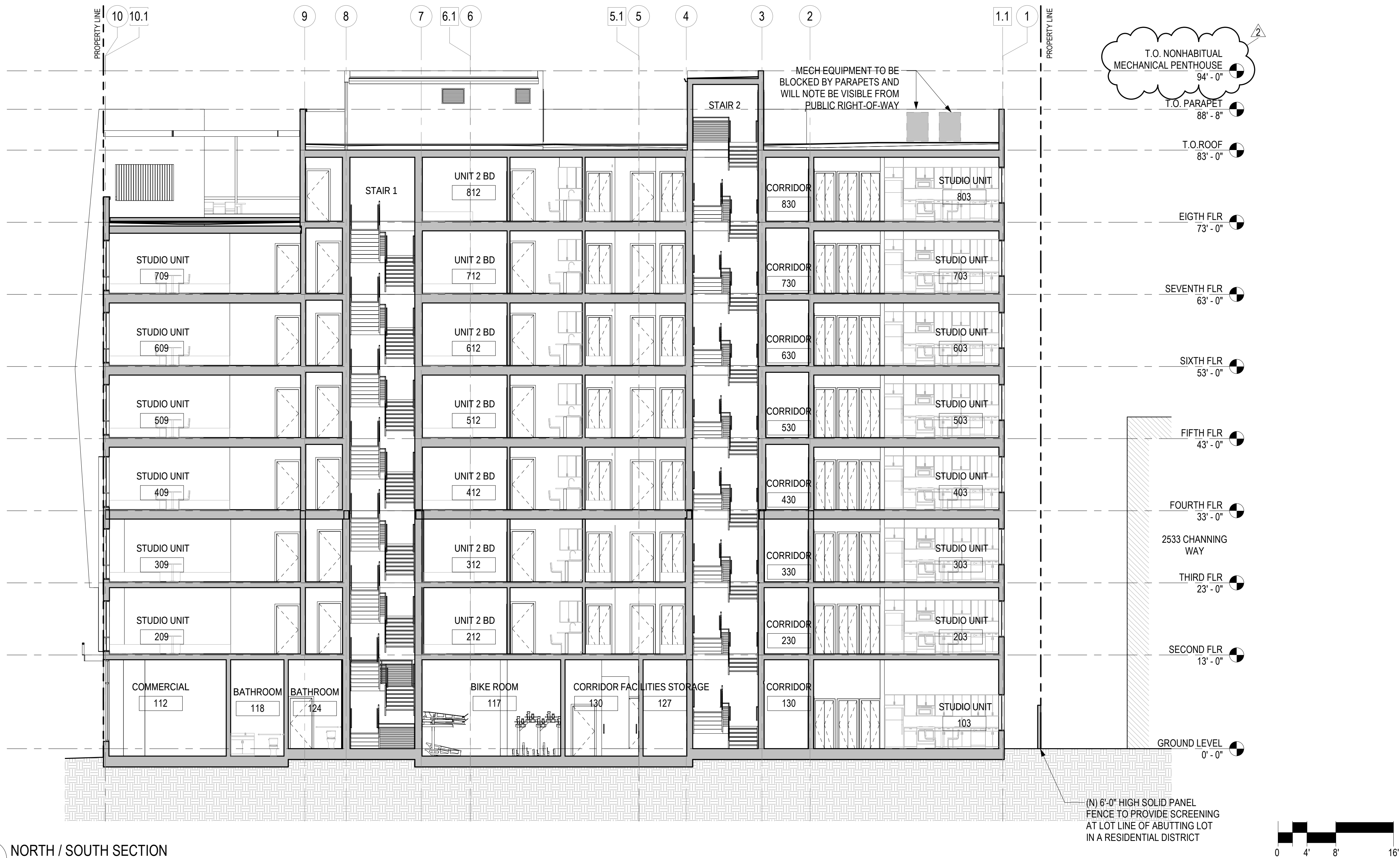
1 NORTH / SOUTH SECTION A302 1/8" = 1'-0" ON 24X36 (1/16"=1'-0" ON 12X18)
