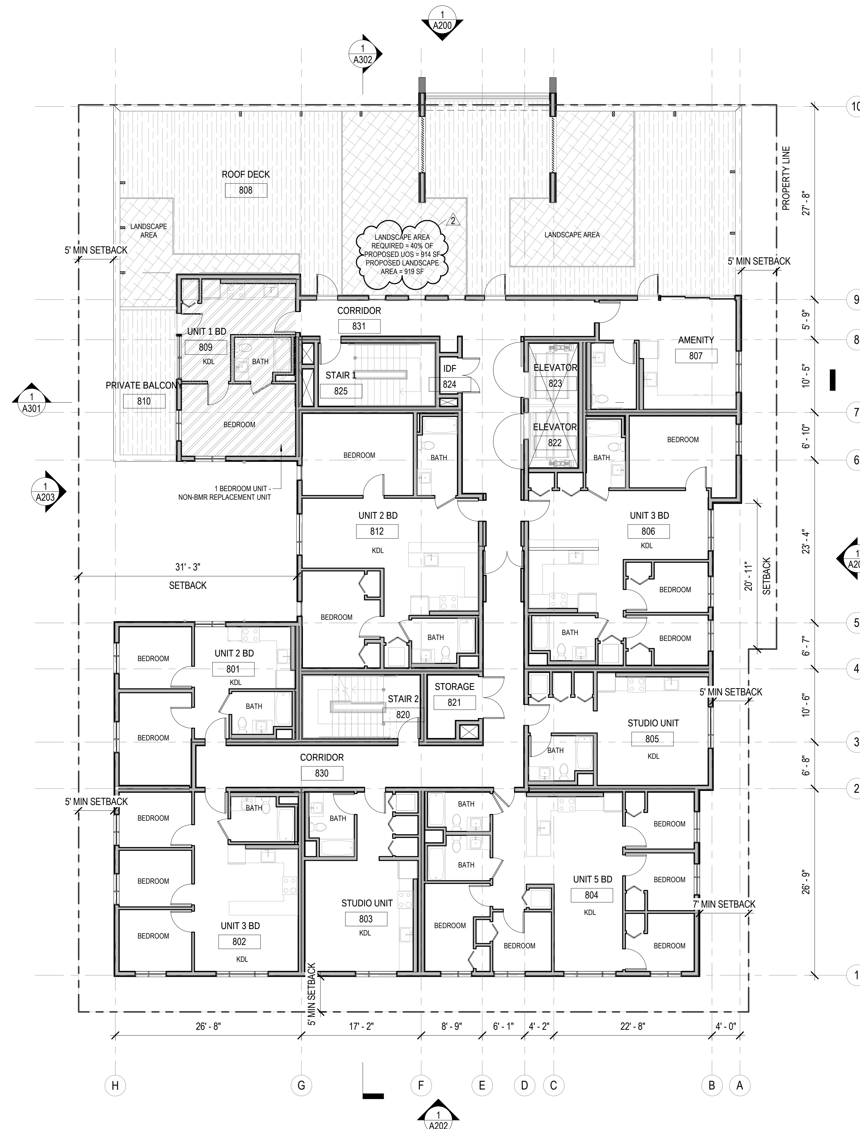
1 EIGHTH FLOOR PLAN A108 1/8" = 1'-0" ON 24X36 (1/16"=1'-0" ON 12X18)
