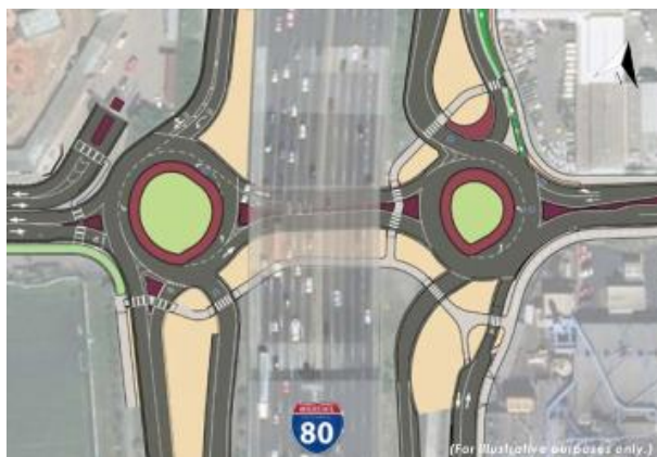
Figure ES-4: I-80 / Gilman Street Roundabout Improvements
