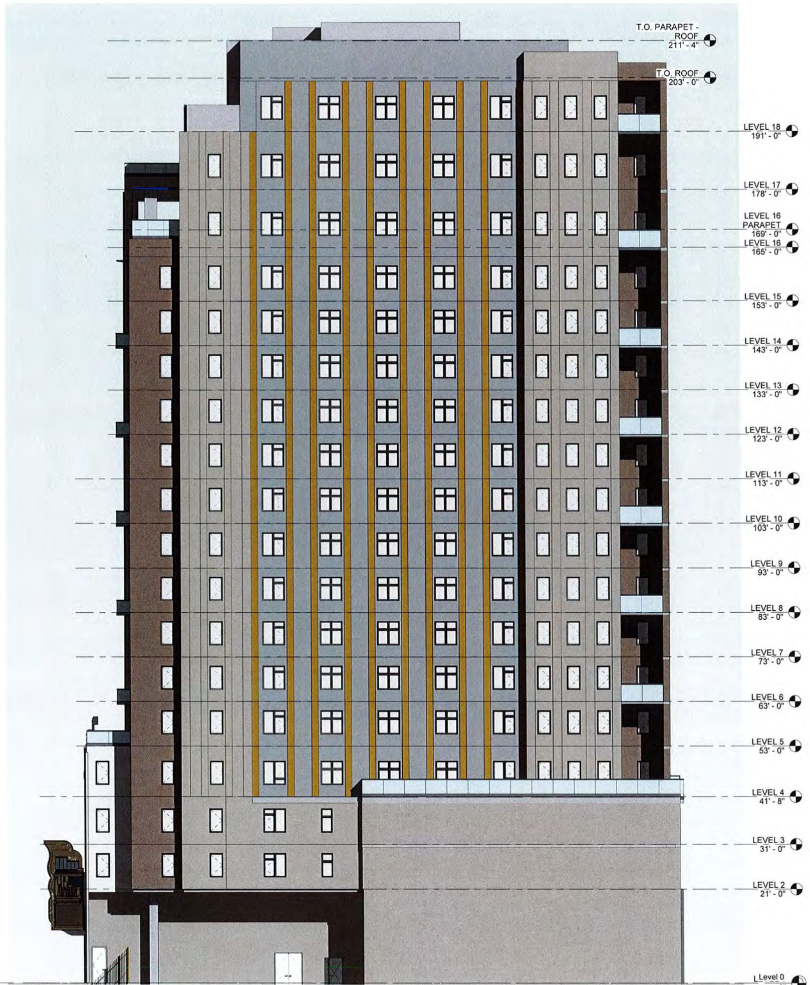
1 EAST ELEVATION A202 3/32" = 1'-0" ON 24X36 (3/64"=1'-0" ON 12X18)
