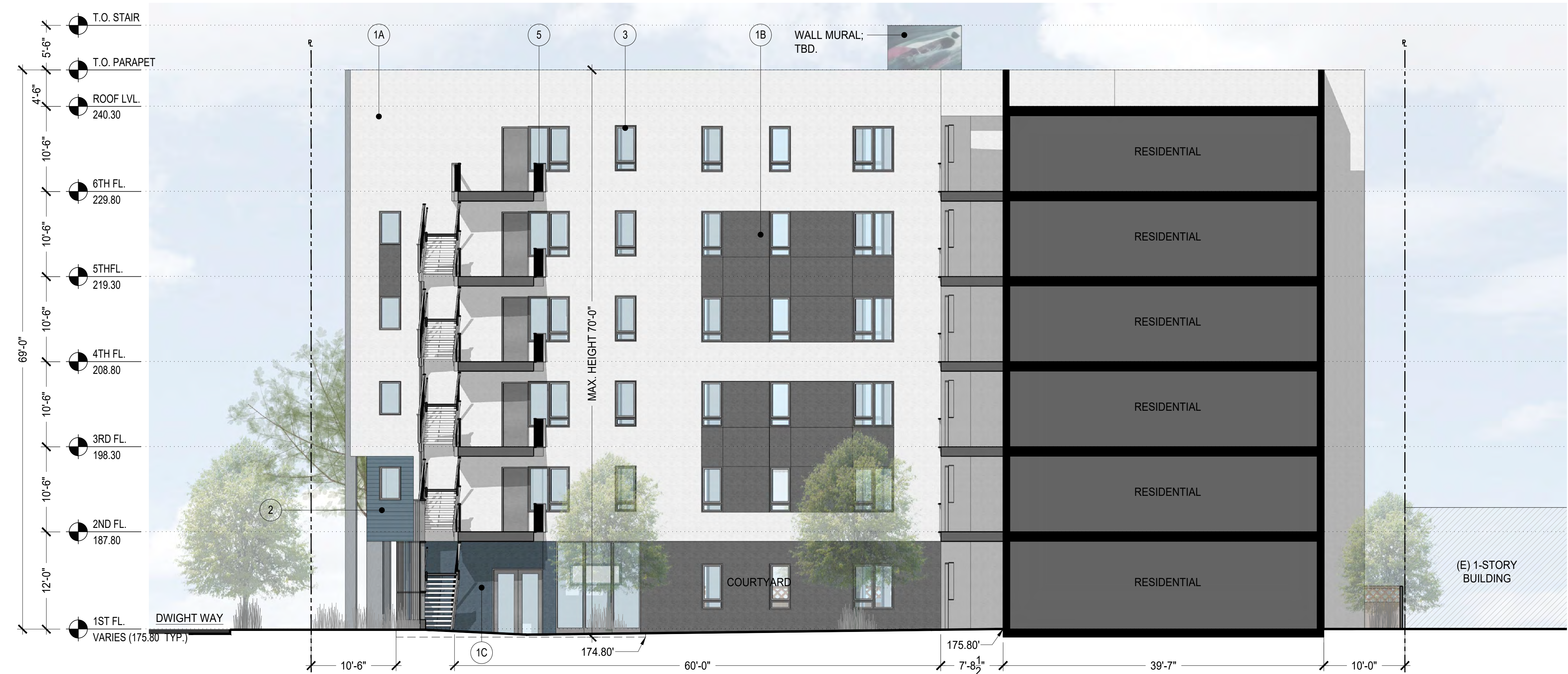
1 EAST ELEVATION - COURTYARD 1/8"=1'-0"
