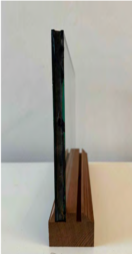
WINDOW REPLACEMENT: NEW CUSTOM WOOD WINDOW SASH TO ACCOMMODATE LEADED GLASS AND NEW DOUBLE PANE GLASS EXTERIOR: GREEN SASH AND REDWOOD FRAME INTERIOR: WHITE SASH AND FRAME
