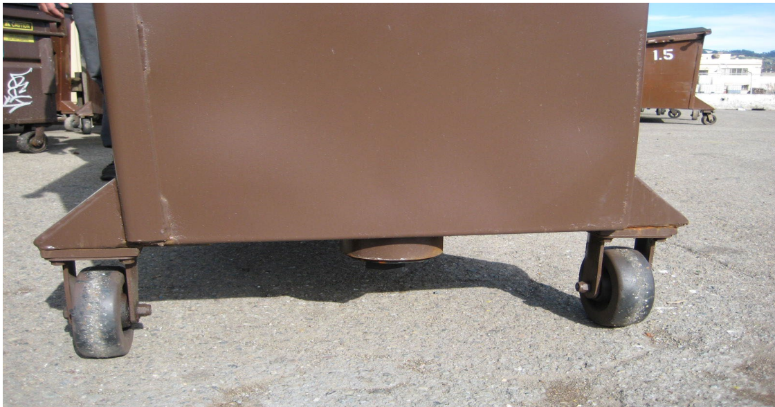
Photo #3 – Example of side view of any container's bottom drain and plug
