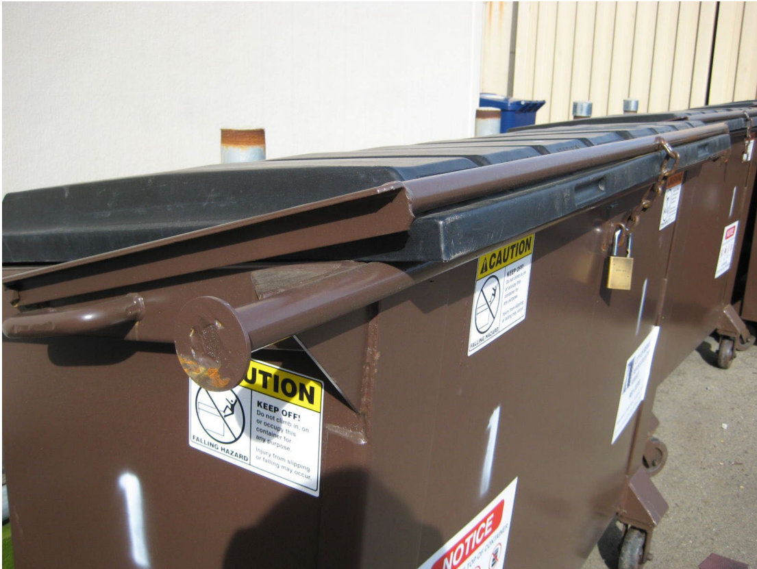
Photo #2 – Example of Rear Loader container lift bar
