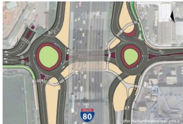
Figure 1-2: I-80 / Gilman Street Roundabout Improvements
