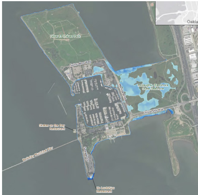
2050 Inundation, Water Level: +10.8' NAVD88 (100-Year Extreme Tide + Low Risk Aversion SLR Estimate), 5-Year CIP Plan.
