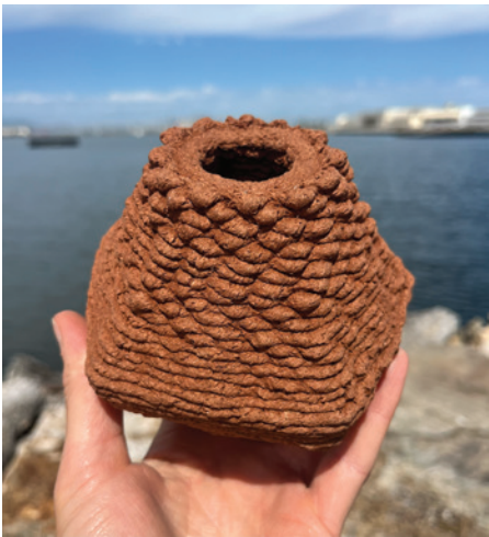
^ 3D printed Wood Adobe made from redwood fiber
