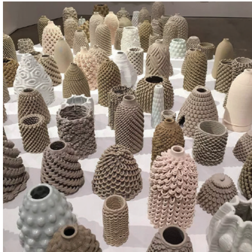
^ 3D printed ceramic texture samples fabricated for Emerging Objects by Alex Schofield.
