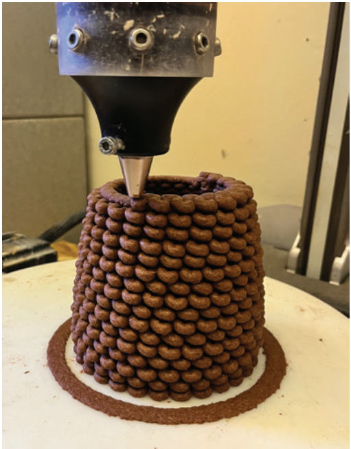
^ Wood Adobe material samples being 3D printed with an extruder at Alex's studio.
