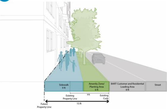
B MLK Jr Way Street Section Diagram (North)
