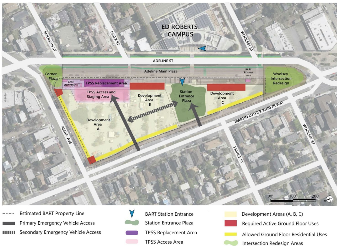
Figure 4. Active Ground-Floor Use Requirements
